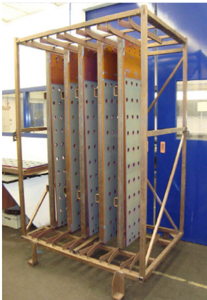
Figure 6 - Tin Insoluble anodes in the rack during coating.
